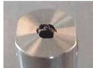
Orifice worn out by slurry
