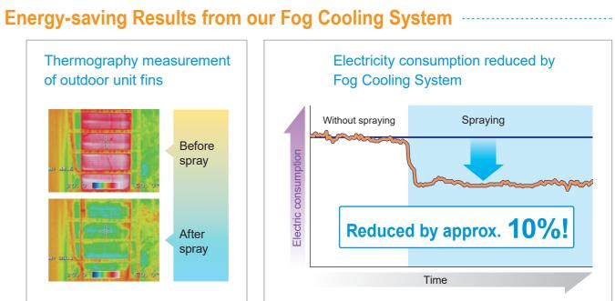
Outdoor temperature: 35°C DB, Indoor temperature: 27°C DB/ 19°C WB Spray condition: Continuous spraying
