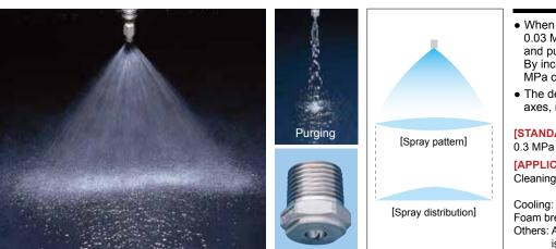
• When the liquid pressure is reduced to 0.03 MPa or lower, the nozzle tip retracts and purges any clogged foreign particles. By increasing the water pressure to 0.2 MPa or higher, normal spraying resumes.
