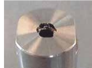
Orifice worn out by slurry
