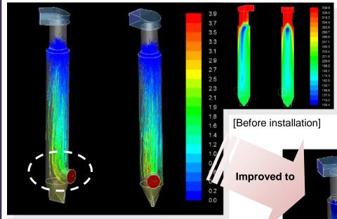
Example of an improvement on the existing gas cooling tower by computational fluid dynamics (CFD) and analysis of nozzles. Flue gas volume: 163,000 m<sup>3</sup>N/hr
