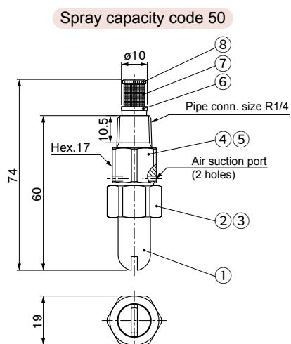
①Nozzle tip ②Cap ③Strainer screen ④Adaptor ⑤Whirler ⑥Strainer holder ⑦Strainer screen (#50) ⑧Strainer cap
