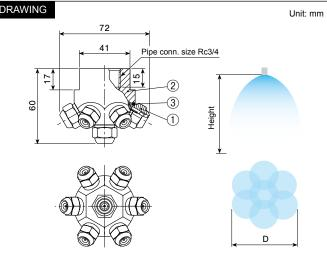
①KB series nozzle ②Adaptor header ③O-ring (NBR) See the chart below for spray dimension D.
