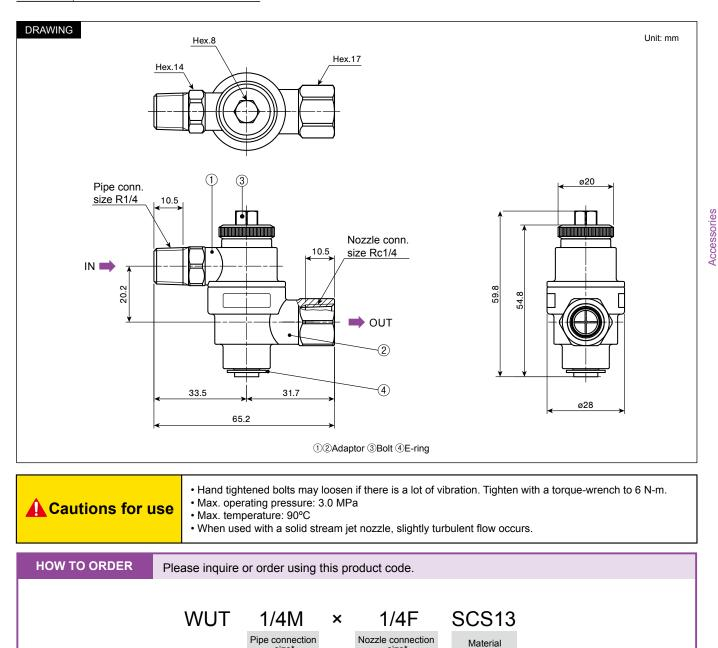
\*"M" indicates male thread ("R" of the ISO standard) and "F" indicates female thread ("Rc" of the ISO standard), e.g. 1/4M = R1/4, 1/4F = Rc1/4.
