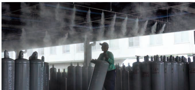
▲Operators tilting and rolling nearly 90-kilogram cylinders into place
