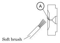
• Use a small ultrasonic cleaner for frequent cleaning or cleaning large quantities of nozzles. Disassemble the nozzle, then clean the orifice disc (#1) and closer (#2).
